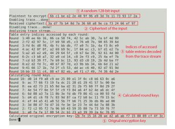
Figure 5: Retrieving the AES Encryption Key.
