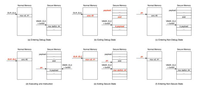
Figure 7: Executing Arbitrary Payload in the Secure State.
