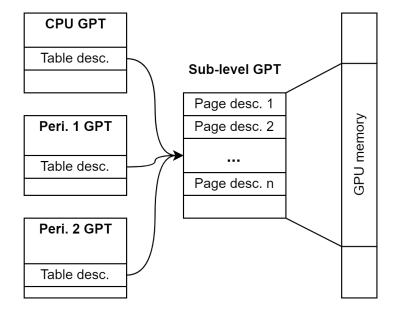
Use the same sub-level GPT to manage access from CPU and untrusted peripherals
