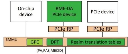
RME-DA focuses on managing PCIe-connected device. Source from Arm DEN0129 manual, version B.a.
