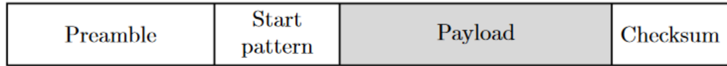
Figure 3: General packet structure of a rolling code. Gray background indicates that the part is either encrypted or authenticated.
